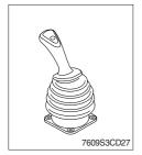
(1) These joystick are used to control the boom and the bucket.
