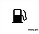
① This warning lamp lights ON when the fuel level is low. Refuel the machine as soon as possible.
