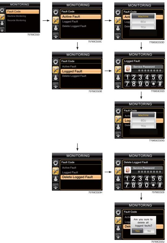
· Monitor the fault code of the Machine/ECU/TCU.
